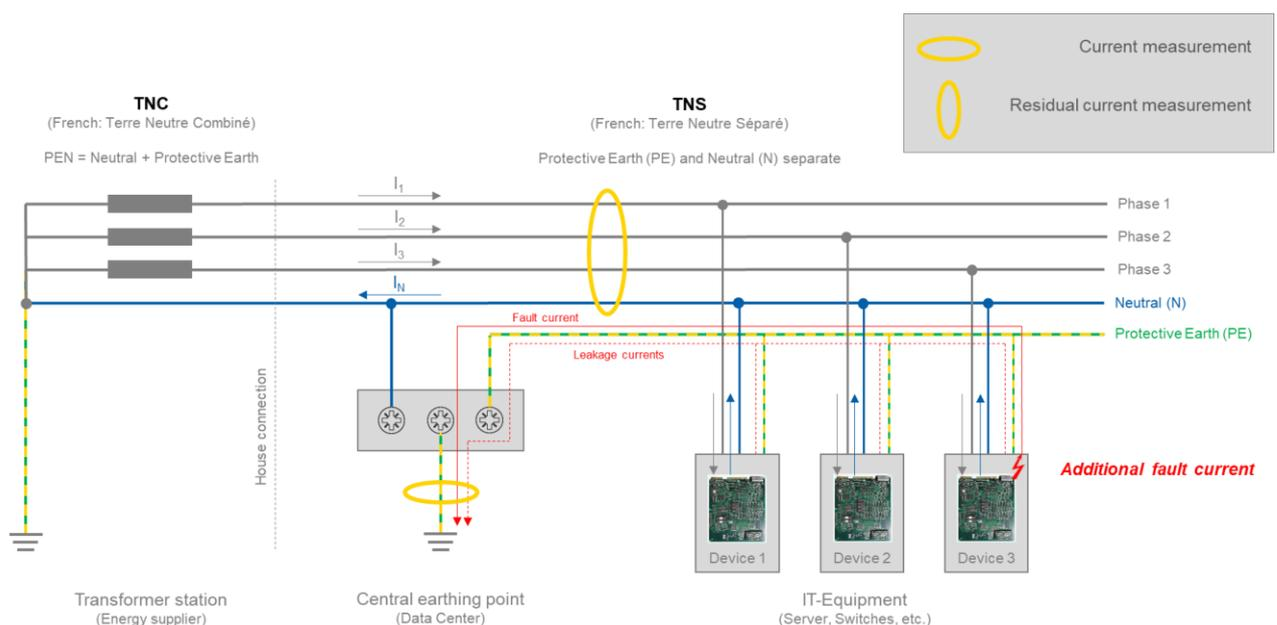
In the first instance, this constitutes a risk to life and limb because the protective conductor actually has a protective function (baseline protection). The responsible electrical manager should therefore take care to monitor these leakage currents.
